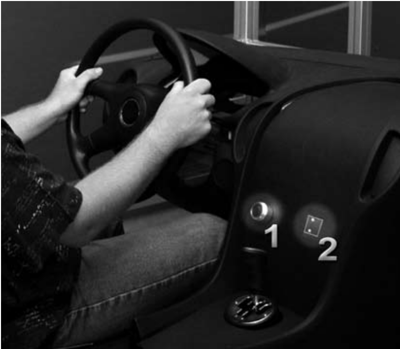
Figure 3: Cockpit design with steering wheel, dashboard and centre console featuring a vibrating, turnable knob (1) and a Peltier element with controllable temperature output (2); actuators can be connected to the components, which can be analyzed with respect to alteration of the driving behaviour within test series
